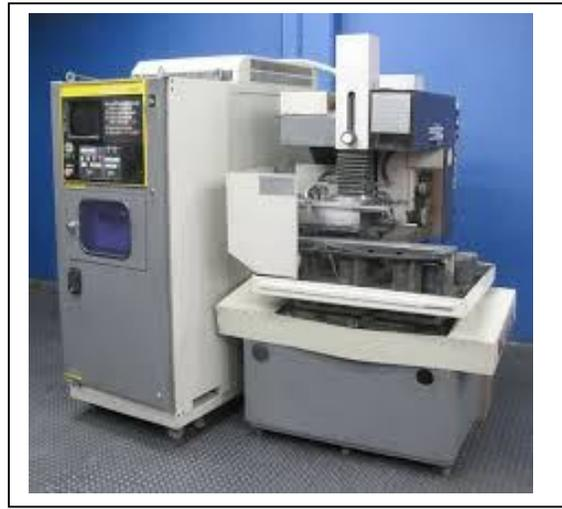
On the EDM machines Tensile Strength comes into play when talking about wall straightness. Even though the wire never contacts the workpiece the process of EDMing creates pressure against the wire from the sparks generated. This causes the wire to lag behind the guides slightly, the less tensile strength the wire possesses the more exaggerated this becomes. It increases dramatically as you increase the part height and forward push of the cut. This can cause a corner washout on the workpiece.
