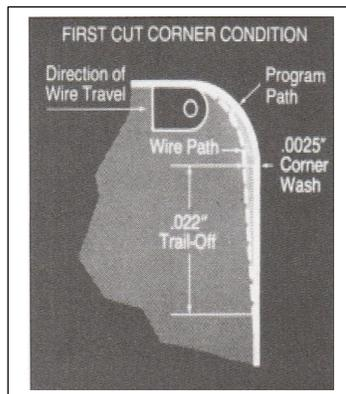
This lag, similar to a truck making a corner, causes the wire to “cut” the corner. This can range from a few tenths on skimming to a couple of thousandths on roughing cuts.
